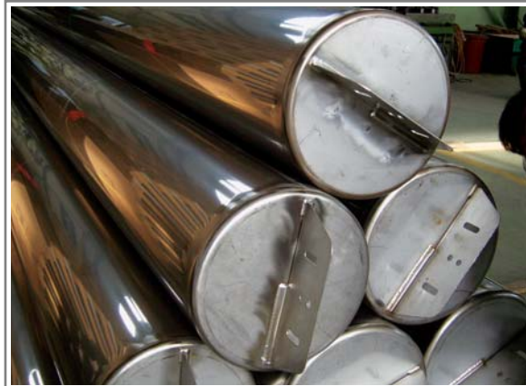
WB Good Finished Pontoon Products for the Final Air Pressure Test Works, 2005 Jan.
