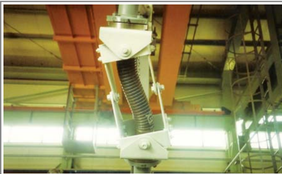
Why do we need twin access type joints? This picture shows the flexible hose must be run lateral direction when the floating deck move vertical position.
