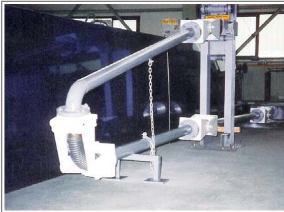
Test Photo for the Pressure & Repeatable Movement Test Over 10,000 Cycles. We believe that this type of test will be worst the operating conditions and expect no trouble to use over twenty (20) Years without drain maintenance works.
